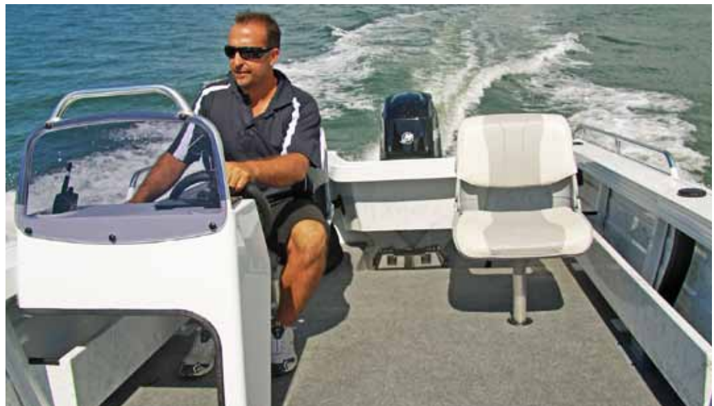
The 460's passenger seat can be mounted aft, allowing increased fishing room.
